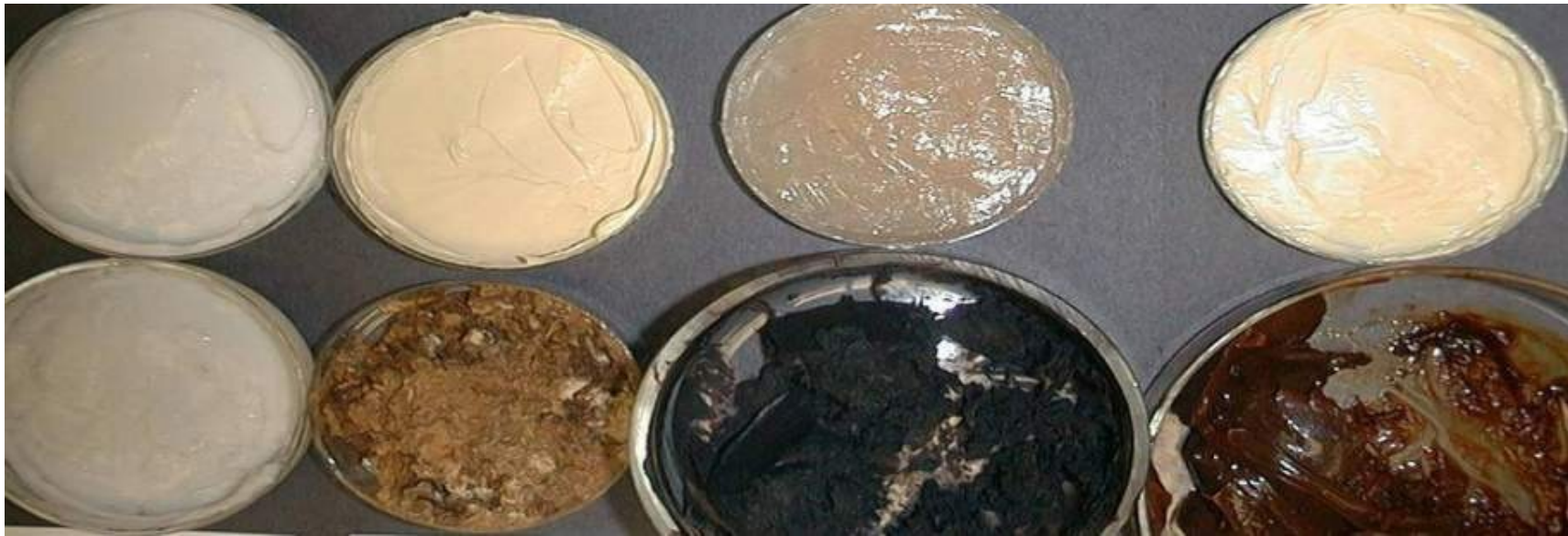
PFPE/PTFE vs. PFPE/Lithium vs. Ester/Clay vs. PFPE/Ester/PTFE/PolyUrea
